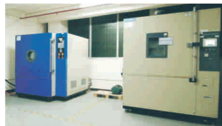
Low Pressure Test Chamber (L) Constant Temperature and Humidity Test Chamber (R)
